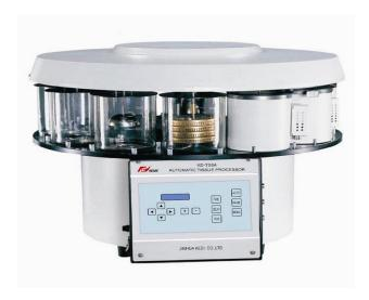
A tissue processor is used to prepare tissue samples for analysis by fixing, staining, dehydrating, or decalcifying them.
