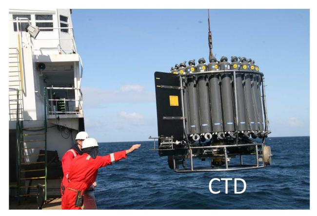
A CTD machine used for measuring the conductivity, temperature, and depth of the salt water it is placed in. This is used to tell the state of the water that animals are swimming in and around to see if it is healthy or to see the living conditions of the animal.
