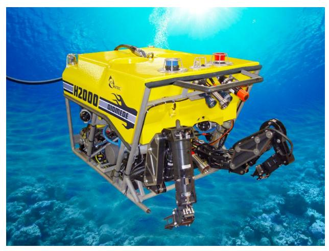
This is an ROV or remotely operated vehicle used for deep sea exploration. Cameras and lights are mounted to the surface to provide a view of waters that humans can not traverse. It is also used to extract samples of minerals and sometimes animals to bring back to research.
