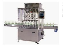
2. Liquid-Filling Machine- This machine is used to fill up liquid prescriptions. This machine fills up the bottle to the right measurements.
