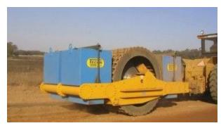
This is a road compactor. As a civil engineer my job is to design and build roads. With this tool I'll be able to compact base and secondary layers of roads to use to put on the roads.
